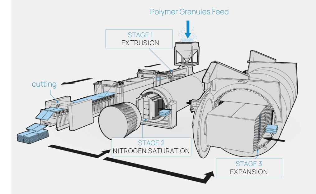
At the heart of what we do is a unique, environmentally friendly three-stage process that uses nitrogen gas to produce a range of premium & high-performance closed cell, cross-linked foams.
