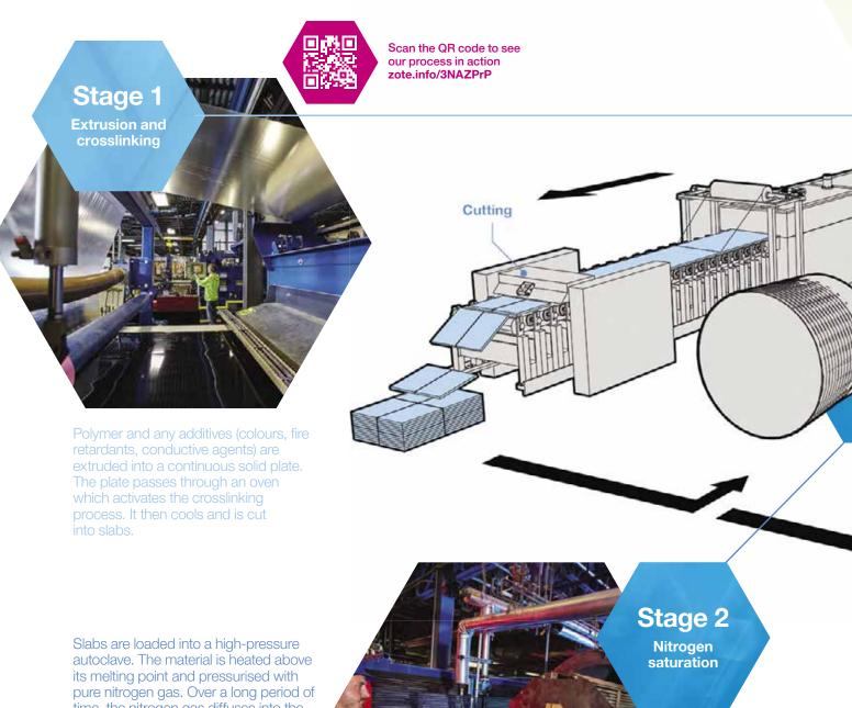
Slabs are loaded into a high-pressure autoclave. The material is heated above its melting point and pressurised with pure nitrogen gas. Over a long period of time, the nitrogen gas diffuses into the slabs. A rapid depressurisation destabilises the absorbed nitrogen nucleating cells in the slab. The slabs are then cooled under pressure in the autoclave, locking the nitrogen in the unexpanded slabs, prior to them being unloaded.
