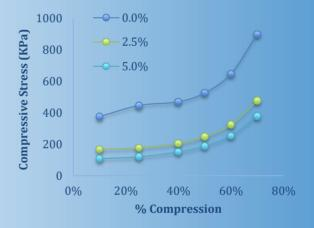
At 0% moisture absorbed, the foam becomes stiff and prone to brittleness. Increasing the moisture decreases the glass transition temperature making the material more ductile.
