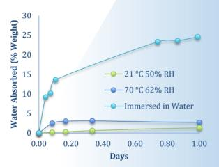
The graph below demonstrates that temperature and humidity affect the rate of moisture absorption.
