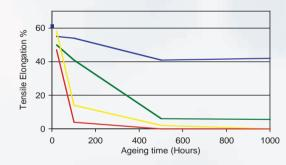
N B50 becomes more brittle when heat aged. This is marginal over a long period of time at 90°C but becomes pronounced at temperatures above this. There is little effect on the strength of N B50 after long term ageing up to 130°C. Loss of strength becomes significant after longer periods at 160°C and above. Moisture will be dynamically absorbed which will improve the ductility of the foam.
