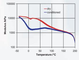
The modulus of N B50 polyamide foam is affected by moisture. When dry, the modulus gradually reduces with increasing temperature until the onset of melting at 180°C when the loss is severe.
