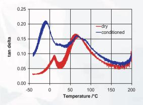
There is a significant increase in damping centred around 60°C. For conditioned foam, there is also significant damping centred around -10°C.
